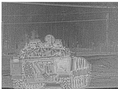
Figure 5.11 DDE set to 100%. The filter functions as an extreme detail booster.
